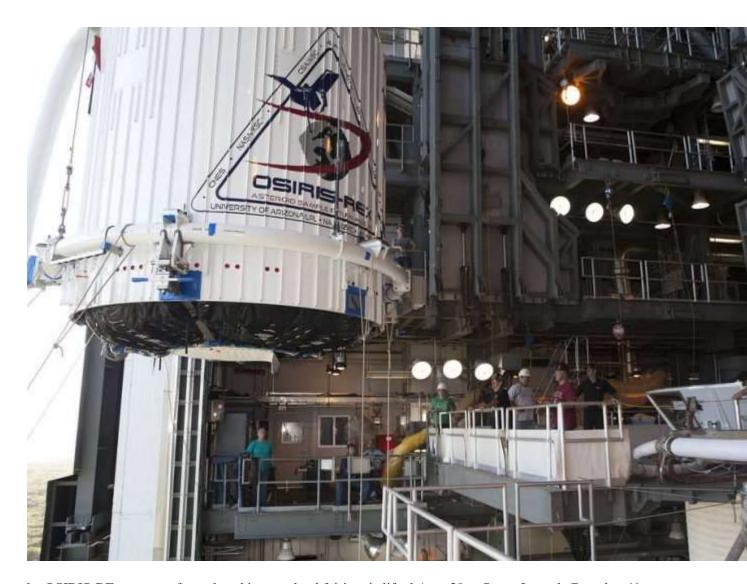
he OSIRIS-REx spacecraft, enclosed in a payload fairing, is lifted Aug. 29 at Space Launch Complex 41 at Cape Canaveral Air Force Station in Florida. The United Launch Alliance Atlas V rocket that is to lift OSIRIS-REx into space was stacked at SLC-41 so the spacecraft and fairing could be hoisted up and bolted to the rocket. Image via NASA/Dimitri Gerondidakis
